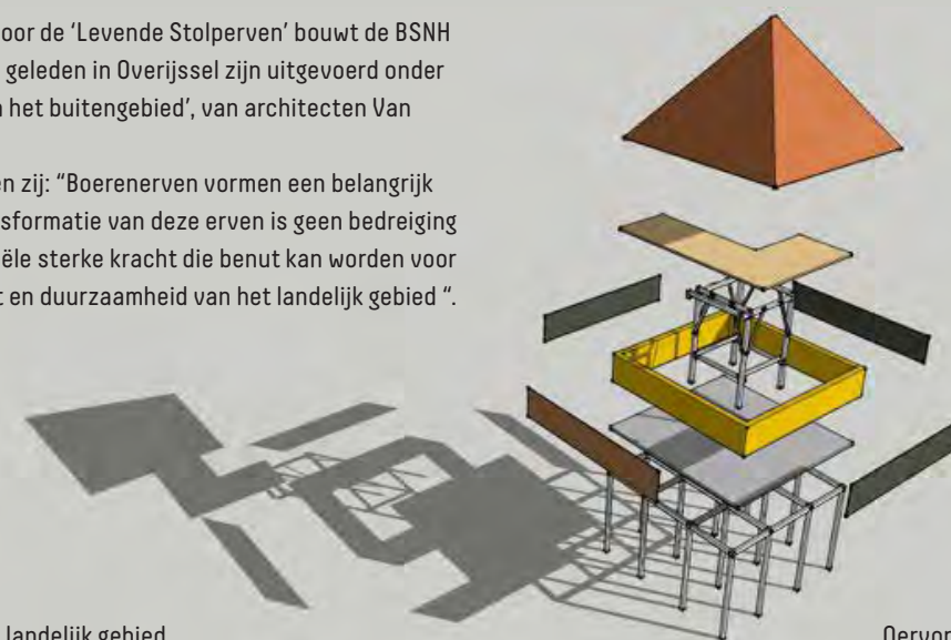
Oervorm stolp, exploded view, Jan-Richard Kikkert
